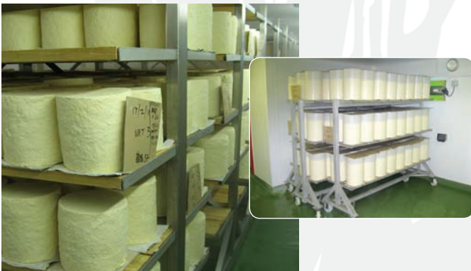
Two types of storage, mobile and tracked racking maximising space.
